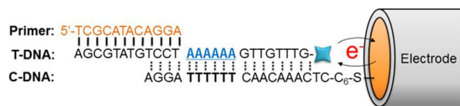
Scheme 2. Schematic illustration to show the oligonucleotide sequences immobilized on the gold electrode surface.
