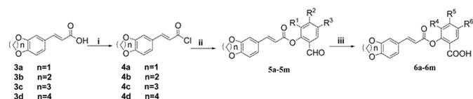
**Scheme 2.** Synthesis of required acids **6a–6m**. Reagents and conditions: (i)  $SOCl_2$ , 80 °C, reflux, 2 h, yield 93–95%; (ii) corresponding salicylic aldehyde,  $CH_2Cl_2$  or ethyl acetate, pyridine,  $N_2$ , ice-bath, overnight, yield 40–60%; (iii)  $NaClO_2$ ,  $NaH_2PO_4$ , 3-Methyl-1-butene, pH 3–4, stirred at rt., 5–6 h, yield 45–60%.
