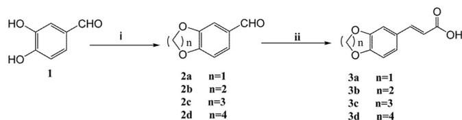
**Scheme 1.** Synthesis of the cyclized cinnamic acids **3a–3d**. Reagents and conditions: (i)  $K_2CO_3$ , dibromoalkane, acetone or DMF, reflux, 4–5 h, yield 50–60%; (ii) malonic acid, pyridine, piperidine, 80 °C, 24 h, yield 70–80%.
